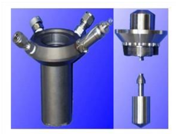
Figure 5-2: High-pressure cell with measuring system. (43)
