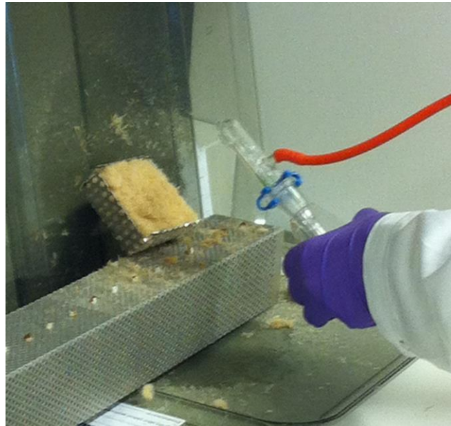
Figure 4.1: Application of the spore suspension using a spray flask.
