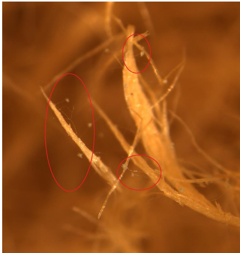
Figure 5.11: Red markings show examples on mold growth observed after 8 weeks in a sample containing TMP1, 3% boric acid and 2% Borax, enlarged 90 times.
