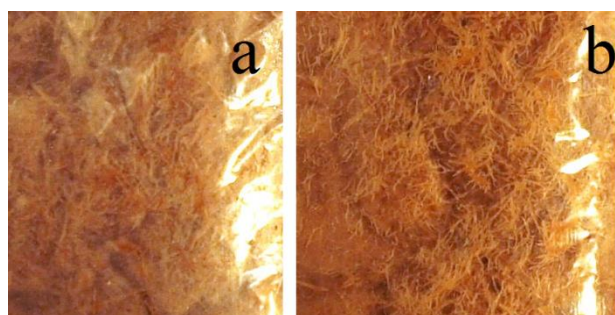
Figure 5.2(a-b): a) A sample of TMP1 without any additives after 1 week of testing. b) A sample of TMP1 added 5% magnesium hydroxide after 1 week of testing. Notice the slightly more orange color compared to the sample in a).
