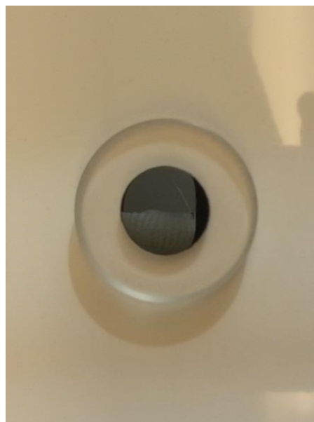
Figure 3.1: Sample holder for the XRD analysis
