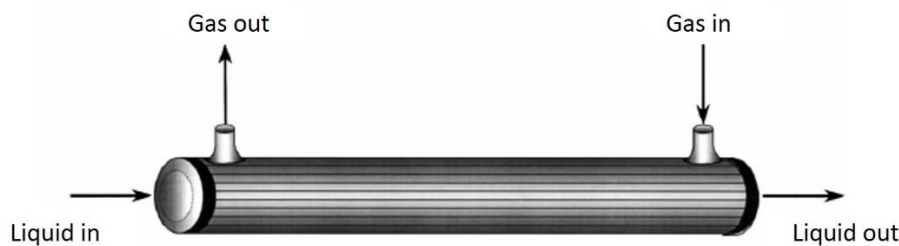
Figure 5-2: Parallel flow hollow fiber gas-liquid membrane contactor (redrawn from [9] and [46])
