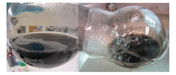
Figure 76 - EXGO and SDS in distilled water. Left picture is before removal of distilled water, Right picture shows the solution during evaporation of distilled water in the rotavapor. The picture shows lot of foam and bubbles.
