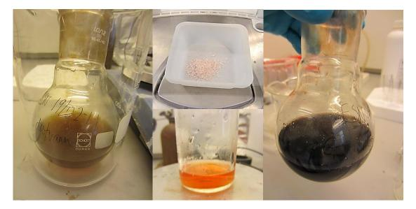
Figure 21- First picture; GO in distilled water. Pictures in the middle; PPDA flakes, and PPDA dispersed in hot distilled water. Last picture; PPDA added to the GO/distilled water solution.
