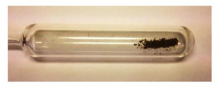
Figure 19 - Custom made glass tube with GO sample before thermal exfoliation [30].
