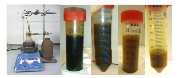
*Figure 16- A: Preparation of GO before washing, B: GO after dispersing in distilled water. C: GO after cleaning in HCl, D: GO after dispersed in ethanol, E: GO dispersed in water [30].*
