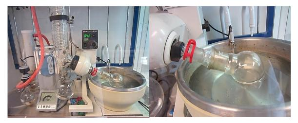
Figure 25 – Epoxy solution in rotavapor for the removal of solvent (acetone).
