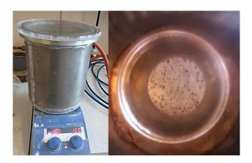
Figure 23 - Vacuum chamber on a magnetic stirrer to the left and epoxy with air bubbles on the right.
