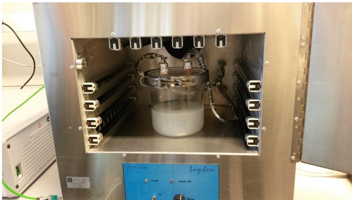
Figure 4: The set up with the reactor inside. Before UVA-exposure (MeOH).
