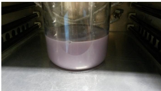
Figure: A2: Reactor with \text{CuTiO}_2 catalyst and 25% glycerin after ~24h of UVA exposure.
