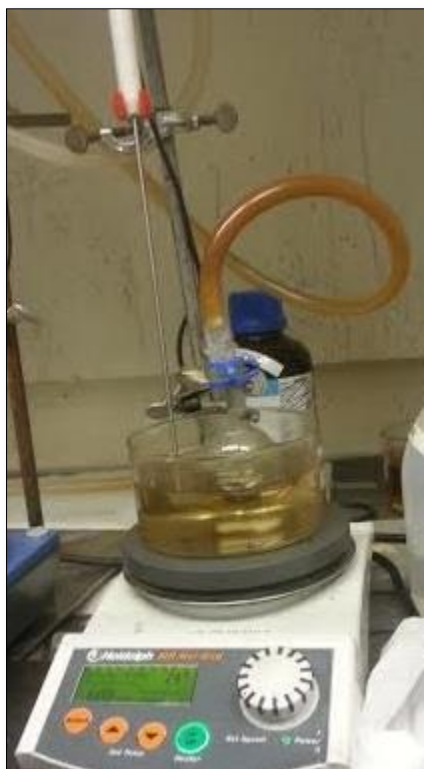
Figure 18 – The setup for the synthesizing of PNIPAm/AAC.
