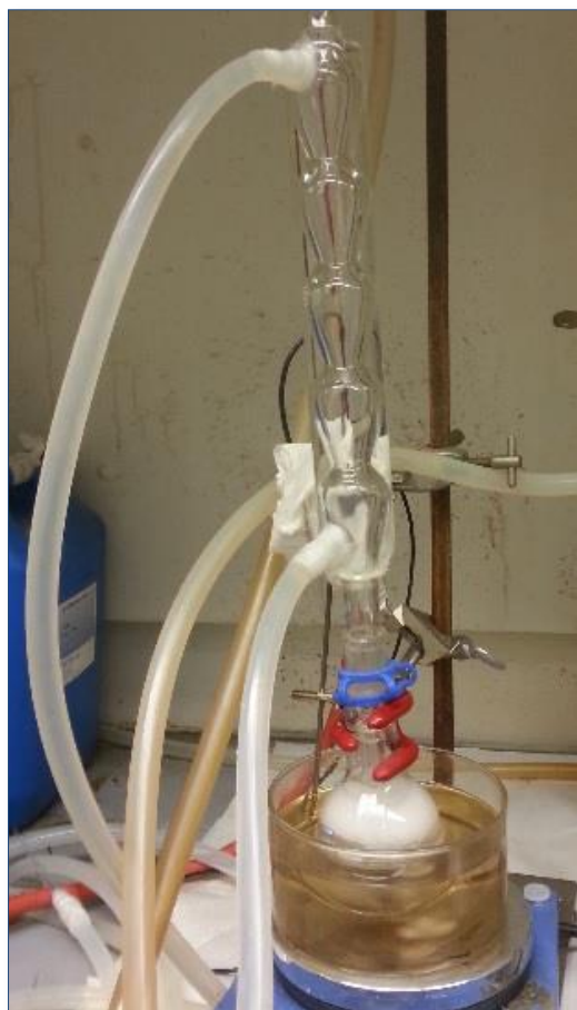
Figure 16 – The equipment used to recrystallize NIPAm.
