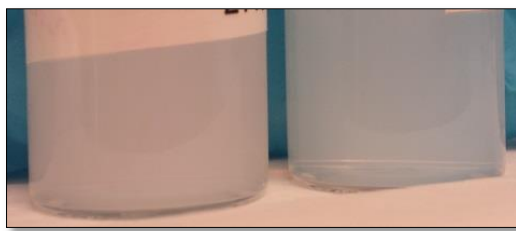
Figure 22 – Shows the difference in color of a solution synthesized with 1.6 mM SDS (left) and 5 mM SDS (right).
