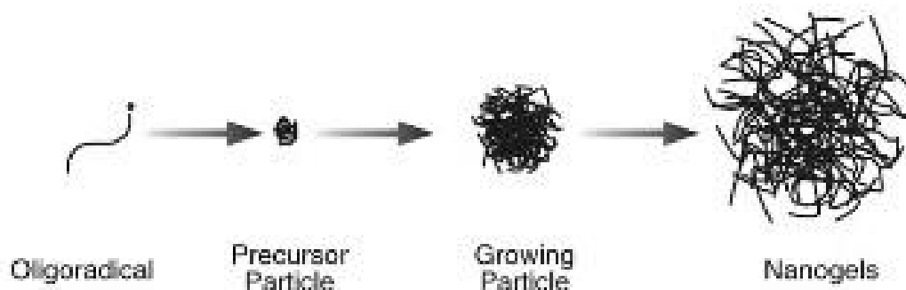
Figure 17 – Principle of precipitation polymerization.[44]
