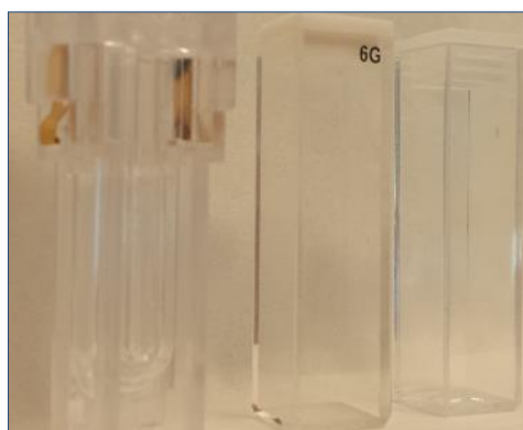
Figure 24 – The cuvettes used in the DLS: The Zeta Potential cuvette (left), the glass size cuvette (in the middle) and the plastic size cuvette (right).
