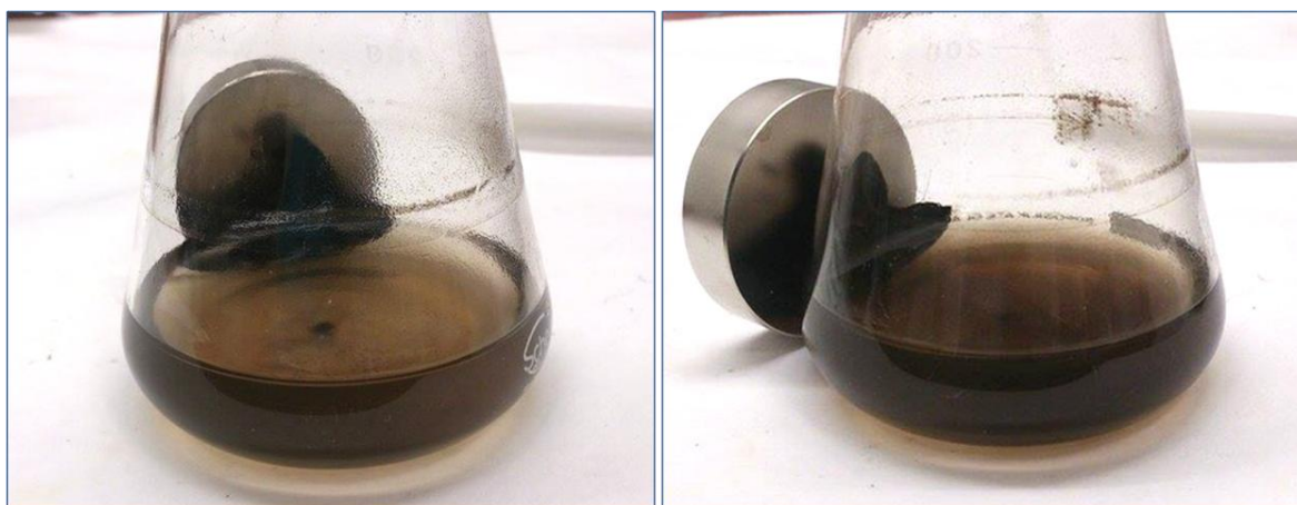
Figure 6-7: The separation of Fe 3 O 4 /SiO 2 MNP and liquid was done by placing a magnet outside of the flask after the silica-coating (SiO 2 MAG1.1).
