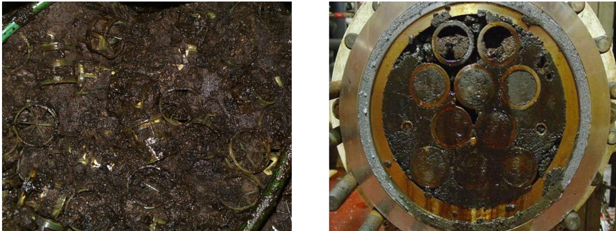
Figure 1-5: Metal naphthenate deposits in flash drum (left) (Mediaas, et al., 2007), and in hydrocyclone (right) (Scaled solutions LTD, 2014).
