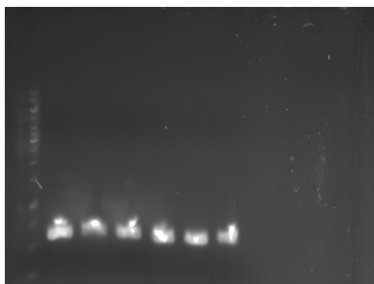
Figure 3.1 - Gel Electrophoresis of the PCR products, obtained from colony PCR for transformants with FPs. DNA 1 Kb Marker, GFPmut3b, EYFP and mRFP1 (Starting from left to right).
