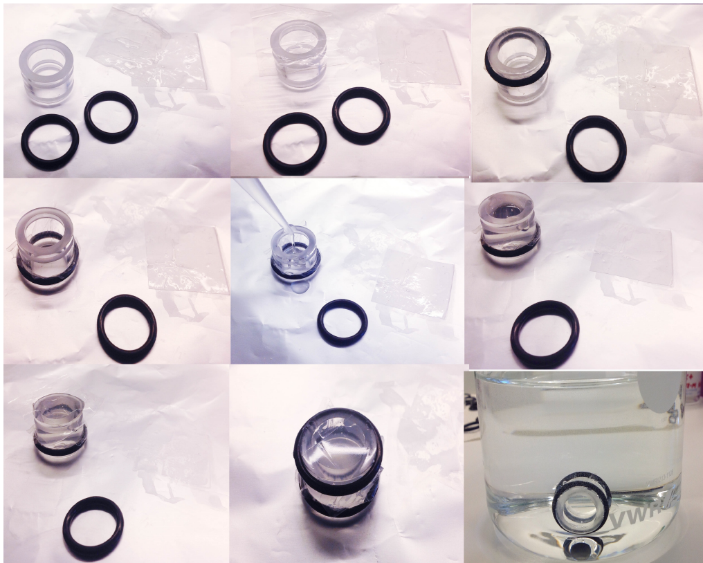
Figure 2.8.1: A graphical overview of the process of making an alginate gel cylinder using cylindrical moulds capped at both ends with a dialysis membrane. The mould is sealed at one end before the alginate solution is added. The other end is sealed before the mould is placed in a gelation bath containing 50 mM \text{BaCl}_2 .
