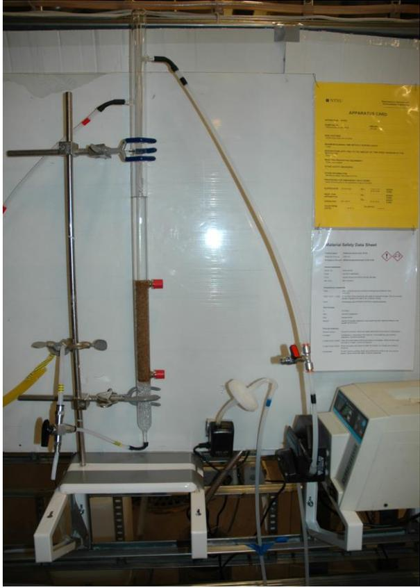
Figure 2.4: Bench-scale continuous flow biofilter.
