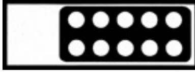
Figure A.1: Teflon coated slide with 10 hybridization wells.
