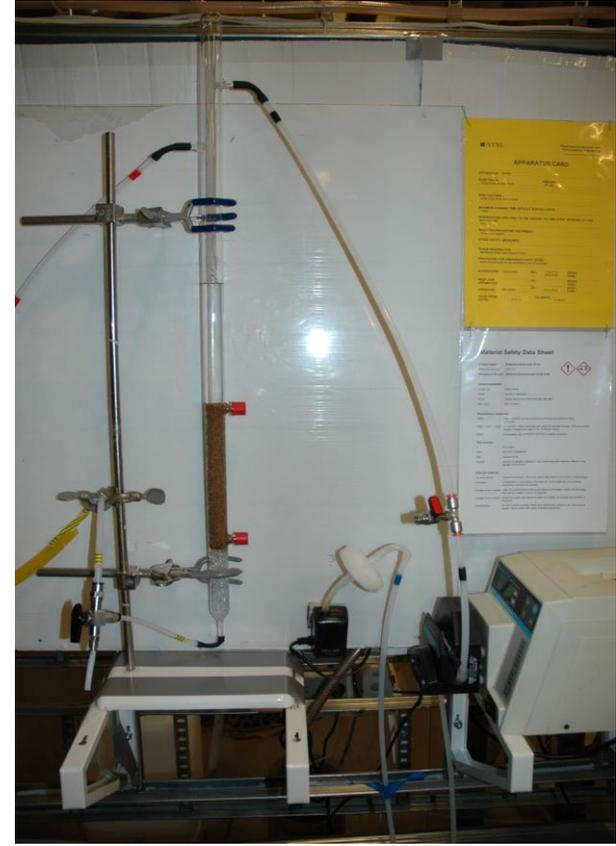
Figure 2.4: Bench-scale continuous flow biofilter.
