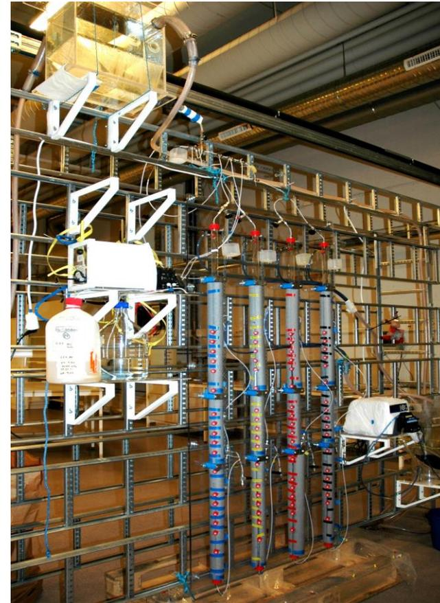
Figure 2.2: Pilot-scale biofilters.
