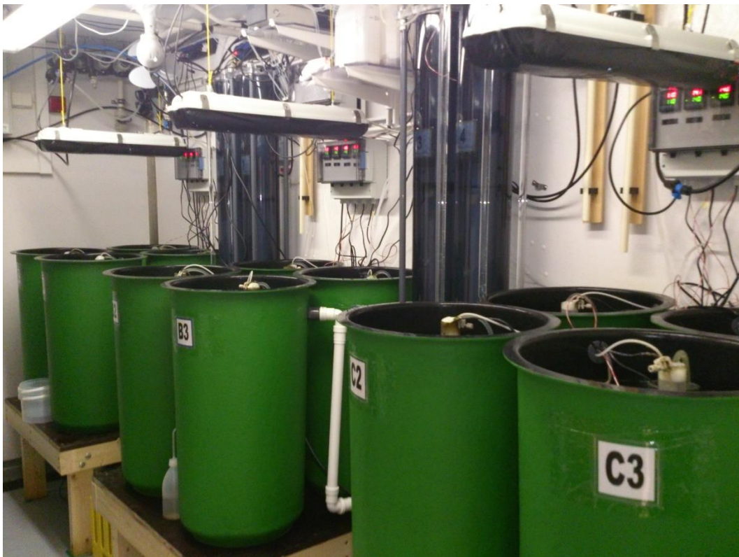
Figure 2.1. A picture of the experimental set up. The copepods were reared in 90 L tanks in three parallels. The temperature was regulated with a temperature controller (mounted on the wall). A temperature sensor and a heat element placed in the middle of the tanks were connected to the temperature controller. The lamps hanging over the tanks simulated sunlight in a 12:12 hour cycle, with light and dark. The CO 2 -enriched air was introduced into the tanks via air stones and distributed from an equilibrium column in the middle. The copepods were continuously feed a mixture of live algae, which was added to the surface.
