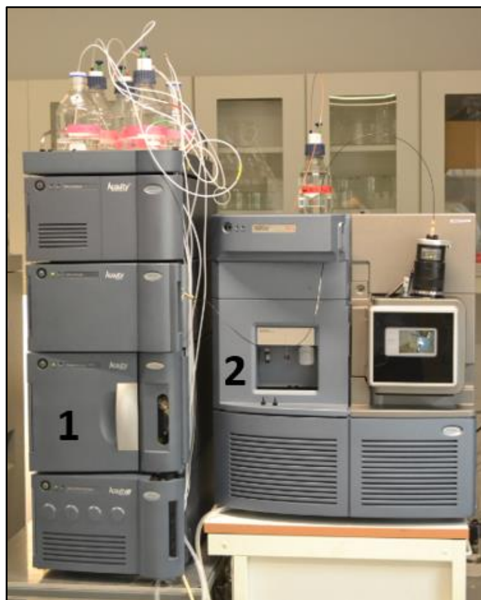
Figure 2.1.2: Xevo™ TQ-S (Tandem Quadrupole Spectrometer with Stepwave ion guide) combined with an Acuity UPLC™ from Waters (Milford, MA), Mass Spectrometry Lab of NTNU. 1) Acuity UPLC; 2) Xevo TQ-S.
