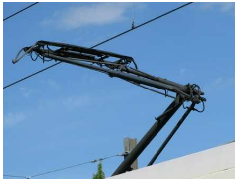
Figure 1.3: Pantograph attached on top of the train, collecting currents from the contact wire ( WordPress, 2010 ).
