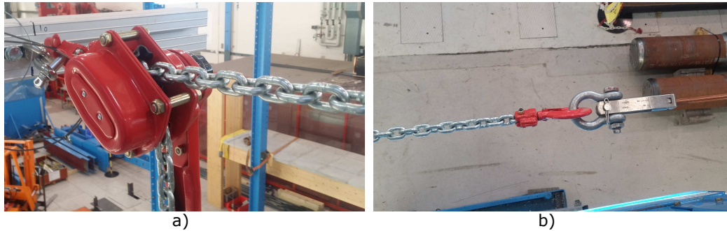
Figure 3.18: a) Jack, b) steel chain connecting the jack to the contact wire.
