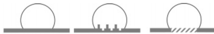
Figure 2.7: The Wenzel and Cassie-Baxter models predict that the CA will change as the surface contact area between droplet and substrate, away from the contact line, changes. However, it has been shown that the CA only depends on changes at the contact line. 45
