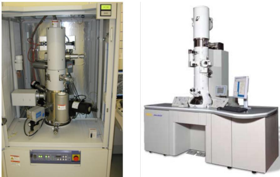
Figure 4.4: The Hitachi S-5500 S(T)EM (left) was the primary characterisation instrument used. A JEOL JEM-2100F TEM (right) similar to the one at NTNU was used for high magnification imaging by TEM. 125, 126
