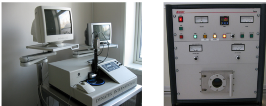
Figure 4.1: The Dynatex DX-III scriber unit (left) was used to scribe samples, while the Diener Electronics Femto Plasma Cleaner (right) performed a plasma clean before metal deposition. 116, 117
