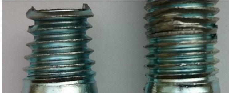
Figure 4.15: Comparison between bolt tests with grip length 124mm and 118mm
