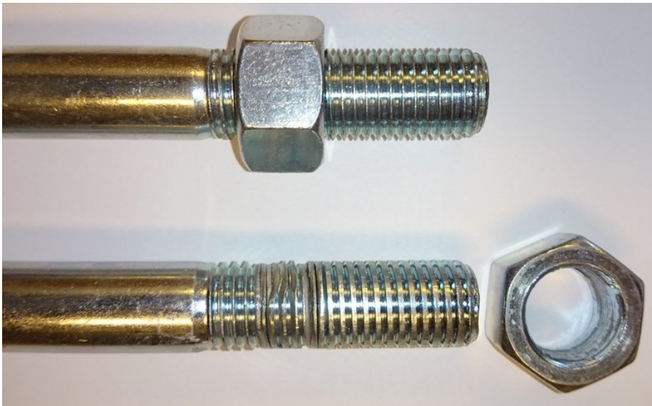
Figure 7.1: Observed thread stripping for test PT-118-01
