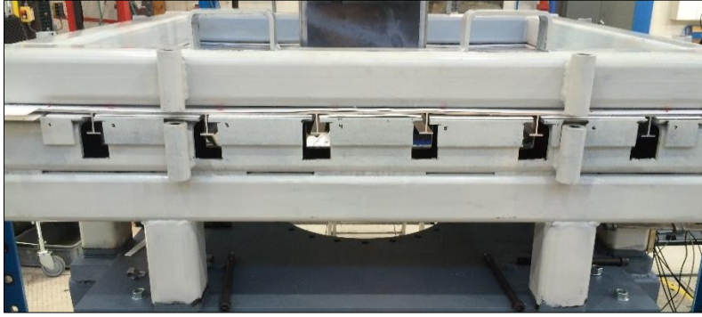
Figure 7-4: Setup of the plate in the rig
