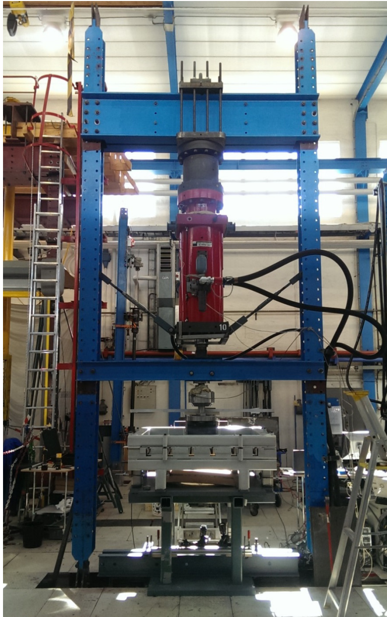
Figure 4-40: Quasi-static test - Support frame installed in test machine.
