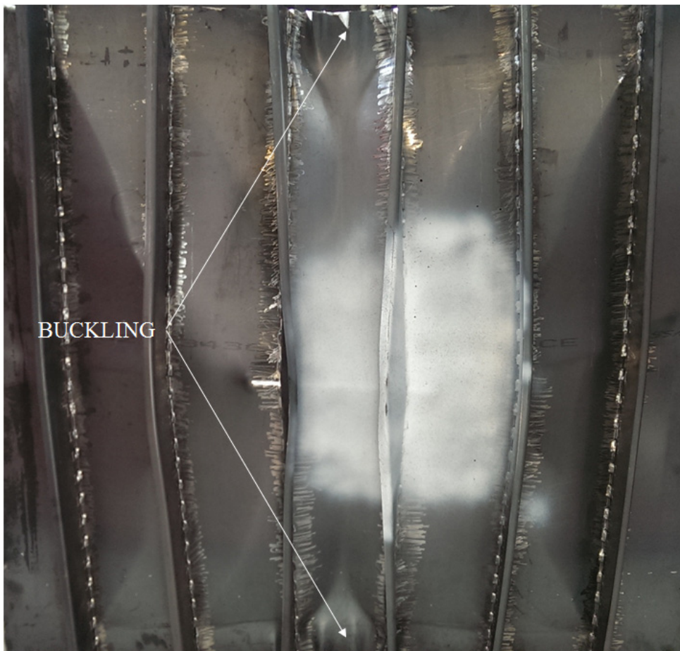
Figure 5-2: Picture of test specimen QSA1 after unloading.
