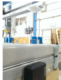
Figure 4-41: Quasi-static test: (a) shows the load cell and attached horizontal bar. (b) shows the ODS pointing on a reference point on the horizontal bar.
