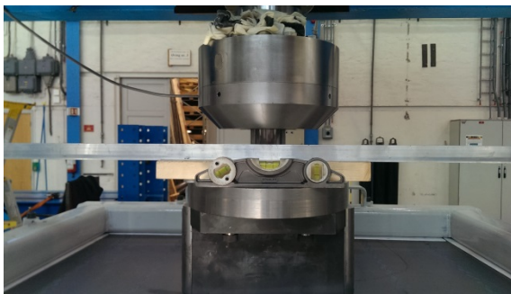
Figure 4-41: Quasi-static test: (a) shows the load cell and attached horizontal bar. (b) shows the ODS pointing on a reference point on the horizontal bar.
