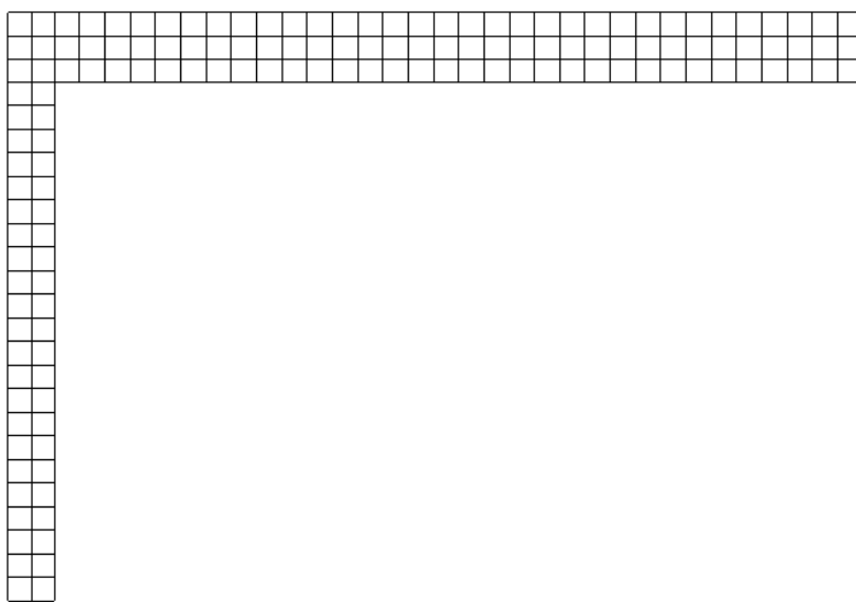
Figure 3.7: Mesh of the model, cut off at the symmetry line through the middle of the beam
