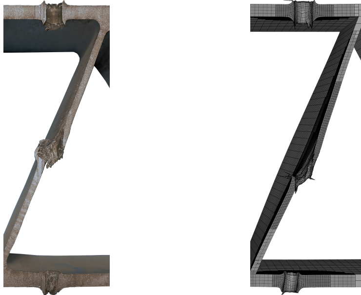
(c) Cross section from shot No. 1 for B95, v_i = 910.5 m/s and v_r = 485.4 m/s (d) Numerical cross section, v_i = 900.0 m/s and v_r = 294.4 m/s
