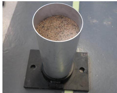
(d) Footing and tube filled with sand
