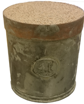
Figure 3.4: 1 liter container used to measure loose and compact sand density.
