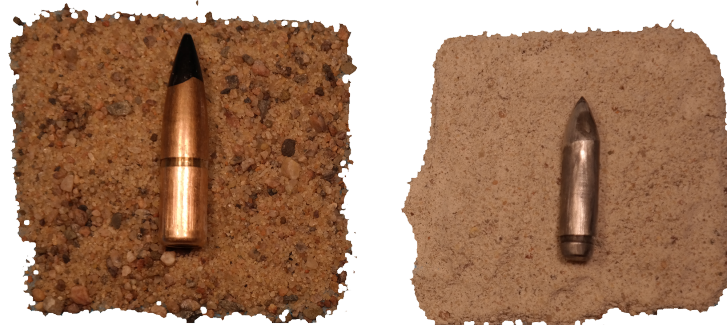
Figure 4.14: Sand and projectile before and after impact, presented for B95.
