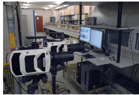
(b) Phantom V1610 high speed cameras
