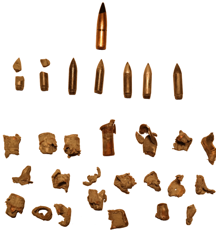
Figure 4.5: Bullet cores and jackets after the testing. Original bullet at the top.
