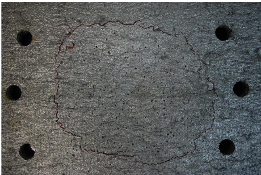
Fig. 62 Failure pattern at the front surface of the foam for experiment "420-1"
