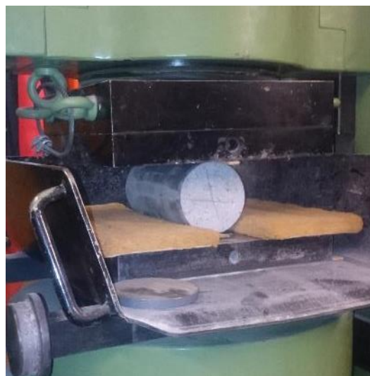
Fig. 46 Experimental set-up of splitting tension test
