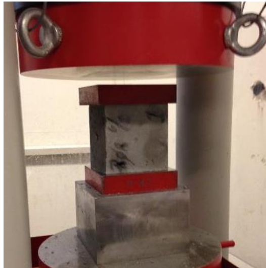
Fig. 45 Experimental set-up for uniaxial compression test
