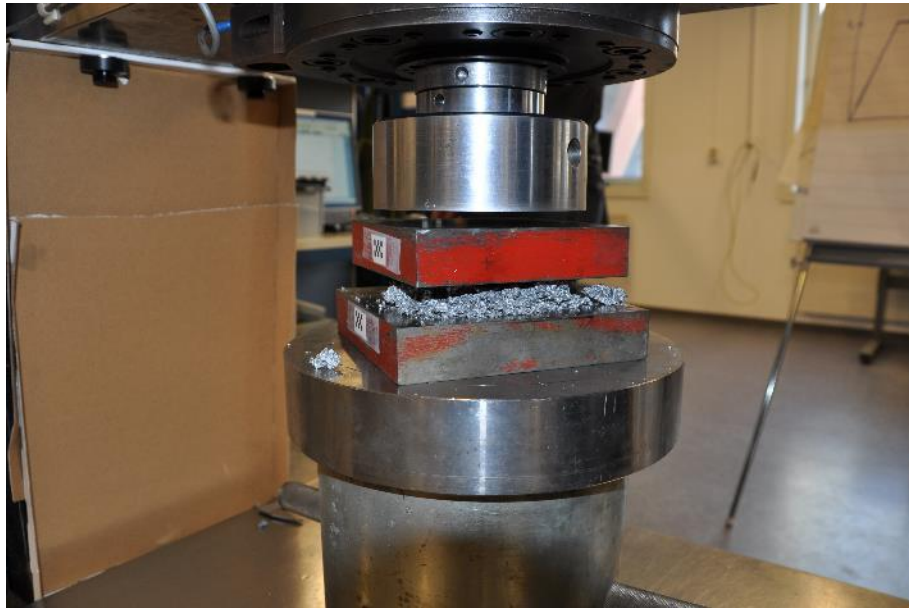
Fig. 36 A test specimen compressed at the end of a test
