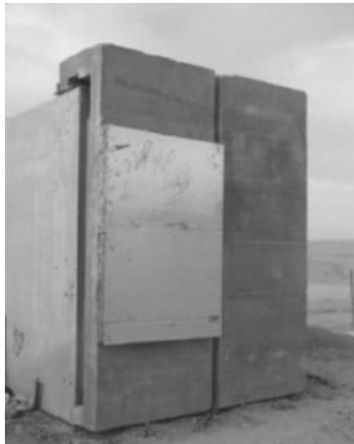
Fig. 2 experimental setup of 3 m span slabs mounted side by side [5]
