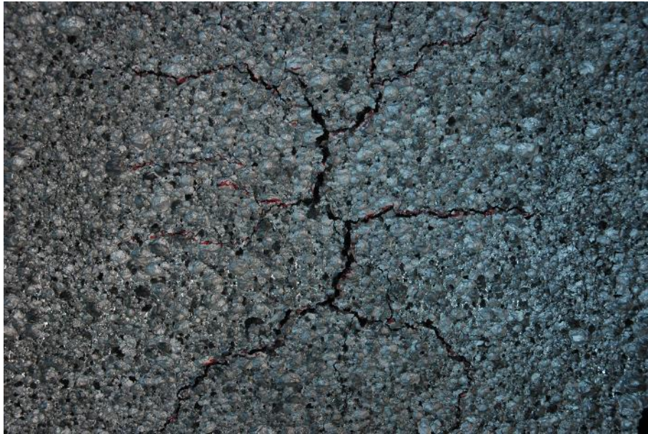
Fig. 61 Failure pattern at the back surface of the foam for experiment "420-1"
