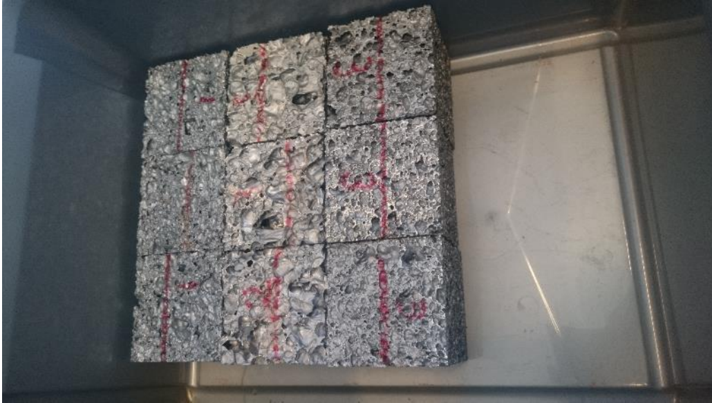
Fig. 32 Aluminum foam test specimens for uniaxial compression test
