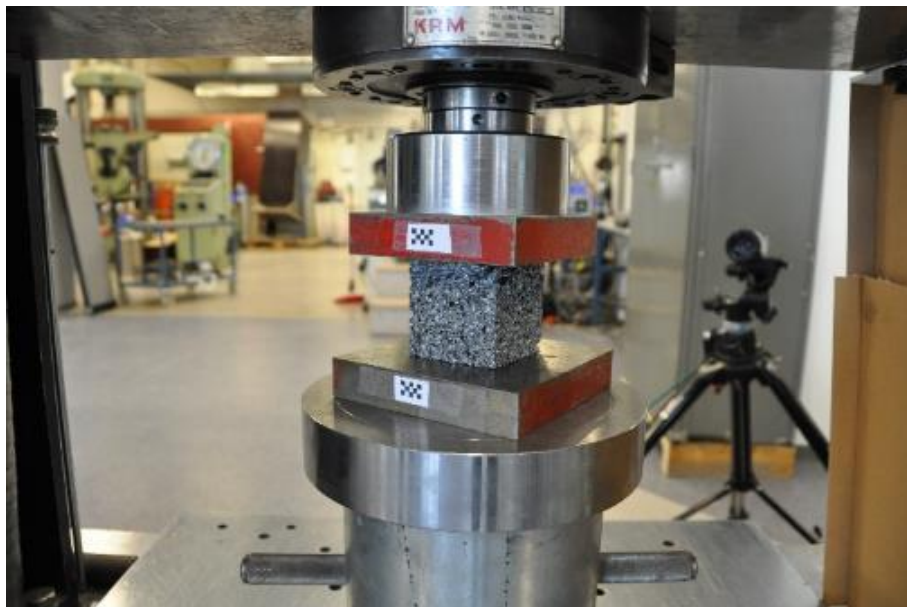
Fig. 35 Experimental set-up of uniaxial compression test of aluminum foam
