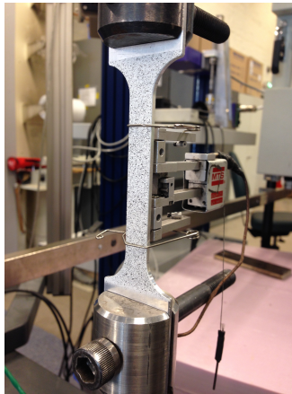
Figure 4.3: Test specimen in the Zwick Roell Z030 machine.
