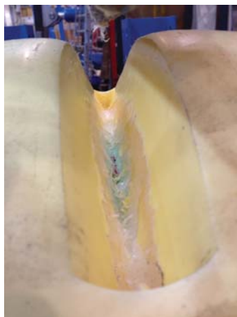
(b) Fracture of the coating
