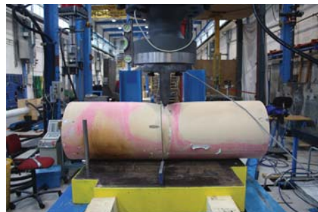
(b) Quasi-static set-up
