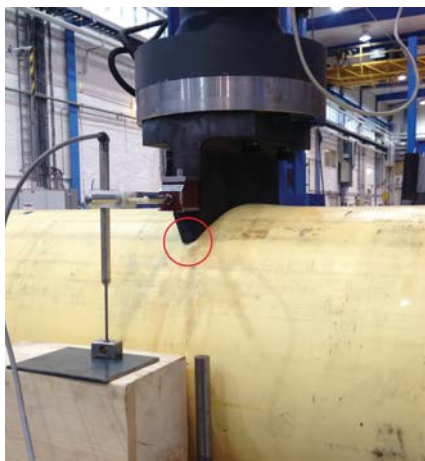
(a) Penetration of the indenter
