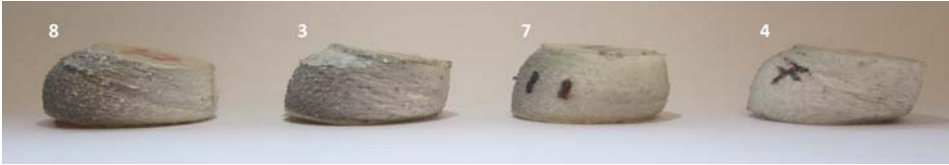
Figure 4.11: Deformation of the 25 mm specimens.
