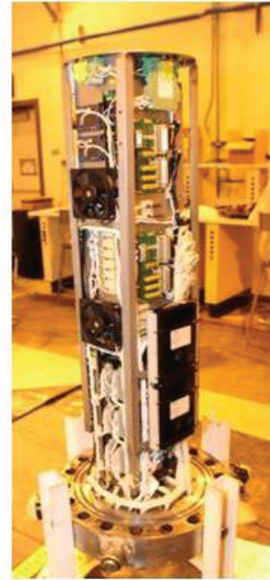
Figure 2.7: Example of a SEM with and without housing, from Engineering Services LP (2014)
