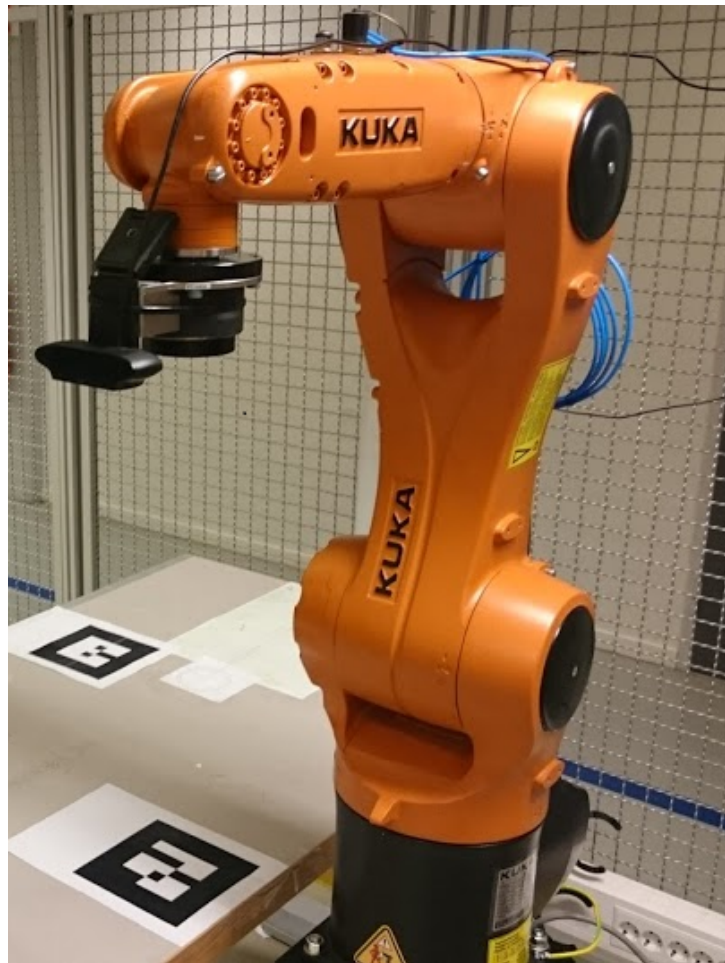
Figure 6.2: Manipulator with a 2D camera connected to end-effector.
