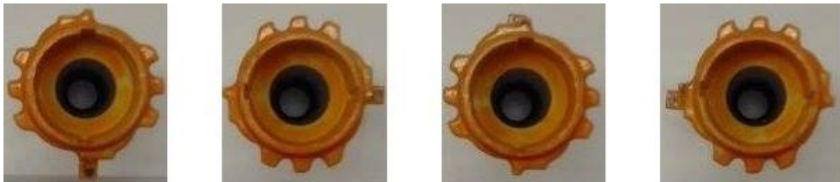
Figure 5.40: From left: The training images I_{o,0} , I_{o,90} , I_{o,180} and I_{o,270} for the piston.
