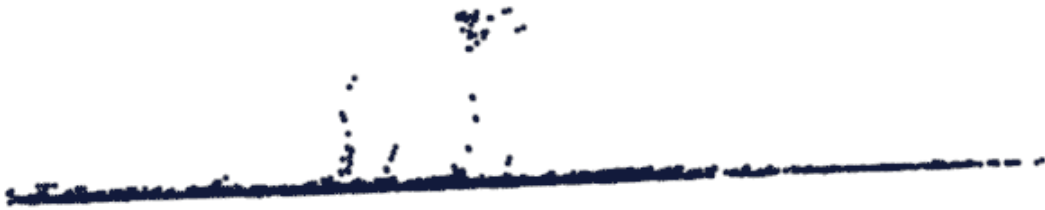
Figure 4.32: Noisy points that are trimmed away by the filter.
