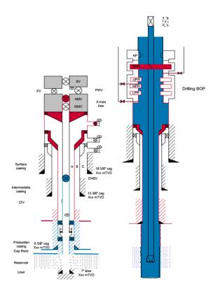
Figure 4.1: Primary and secondary barriers in production and drilling mode (Standar Norway., 2004)
