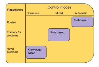
Figure 3.2: Location of the three performance levels within the "activity space" defined by control modes and situations (Reason, 1997).
