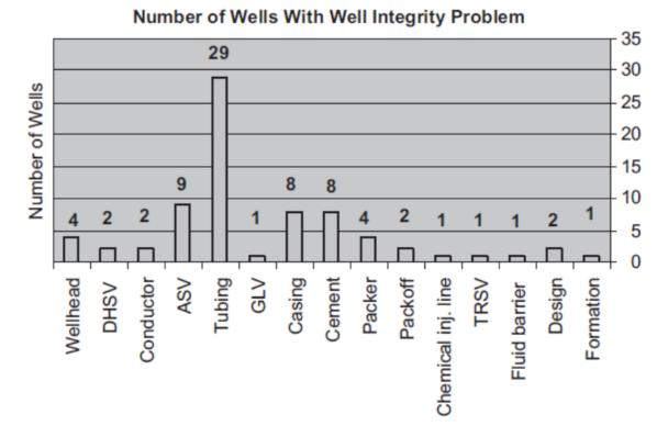
Figure 4.2: Number of wells suffering from different barrier element failure. (Vignes and Aadnoy, 2008)
