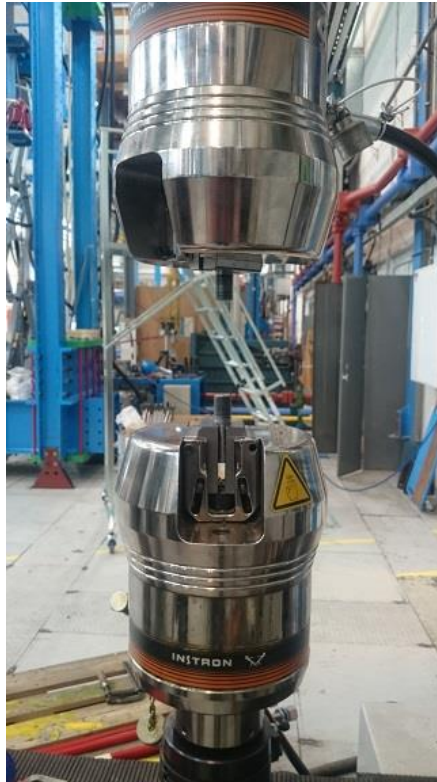
Figure 18: Adhesion test setup
