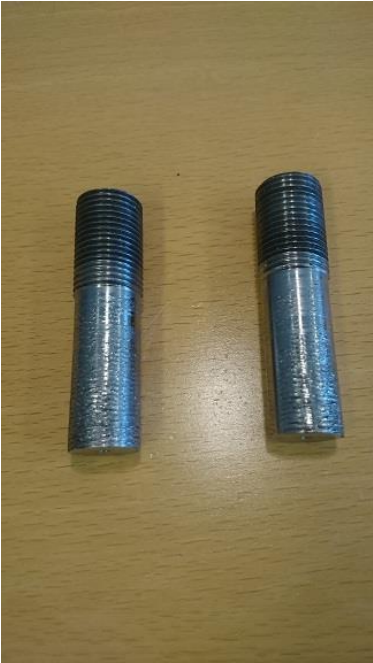
Figure 16: Adhesion test adapters
