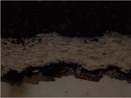
Figure 51: Sample 1 cross-section at 50x magnification, adhesion loss
