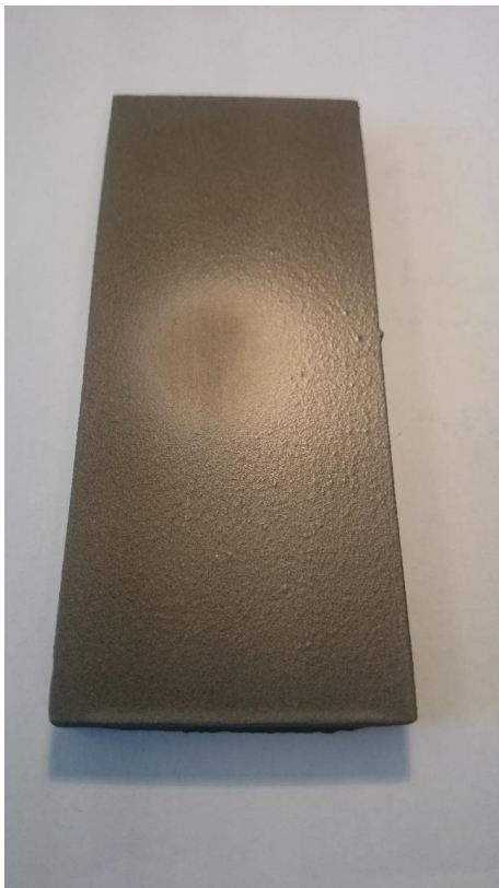
Figure 56: Sample 2 after erosion test
