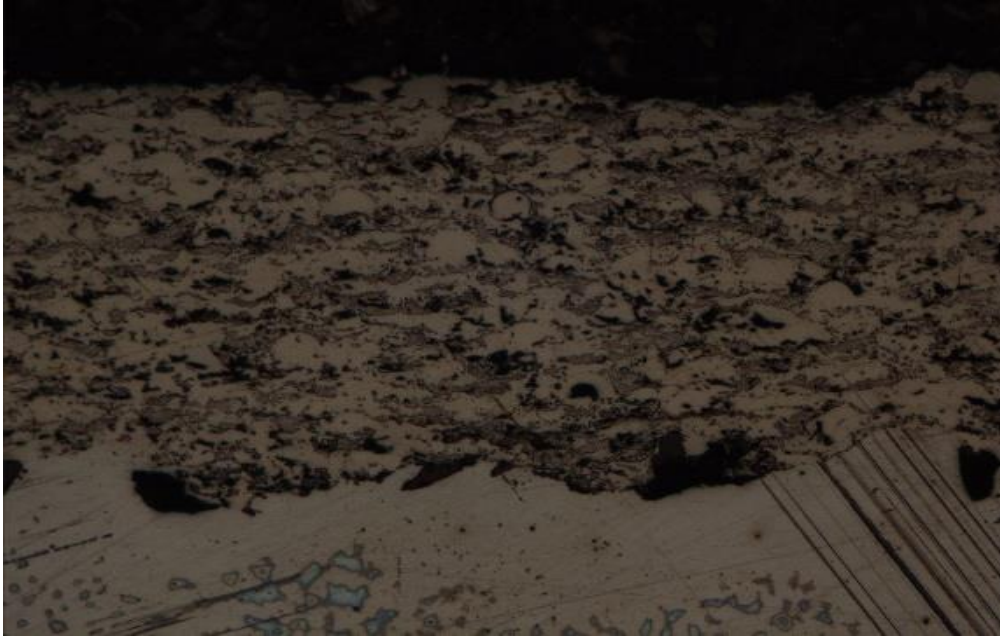
Figure 23: Microstructure of 90 degree spray at x100 magnification
