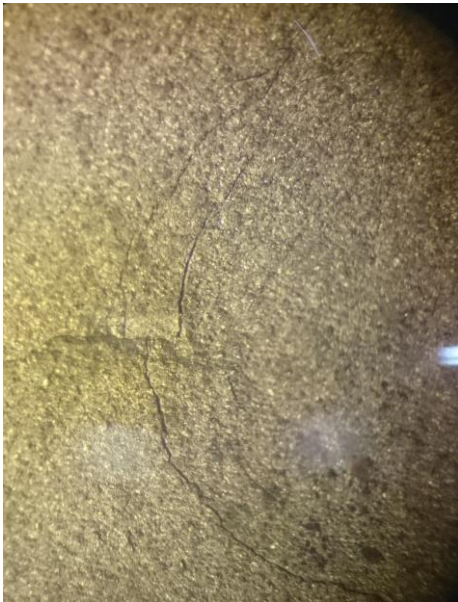
Figure 43: Cracking pattern for impact test
