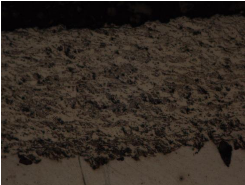
Figure 22: Microstructure of 45 degree spray at x100 magnification
