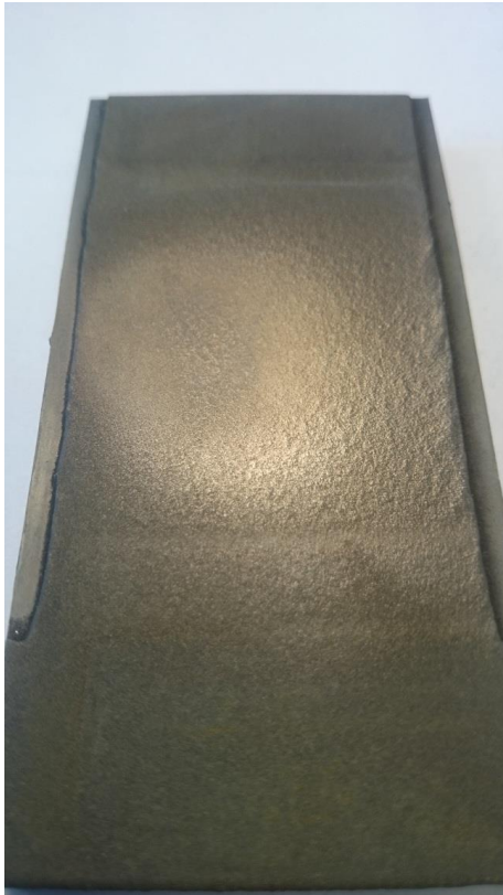
Figure 55: Sample 1 after erosion test
