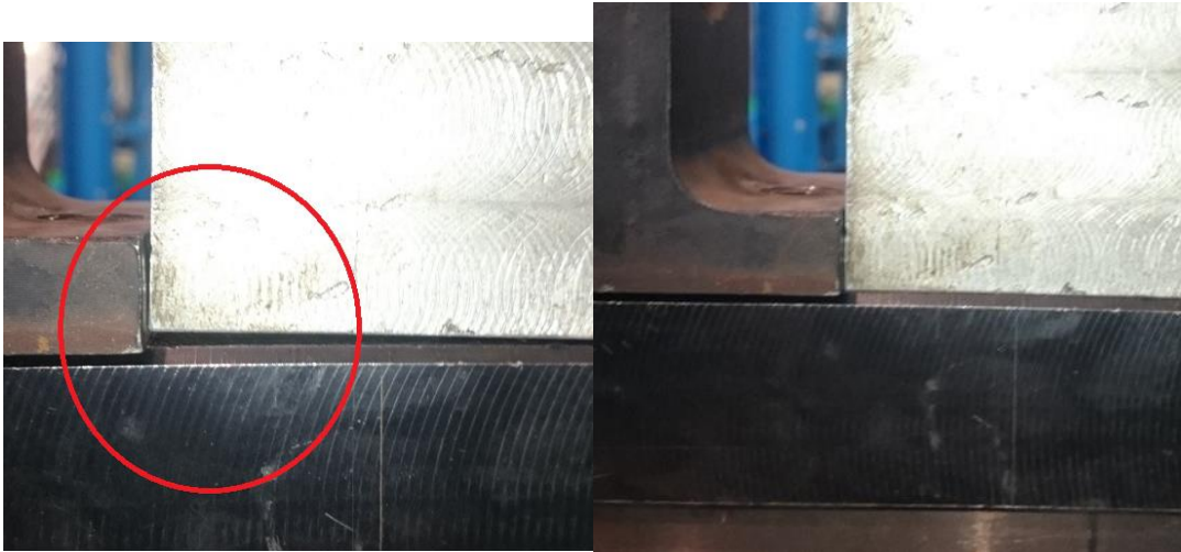
Figure 40: Support movement during bending test
