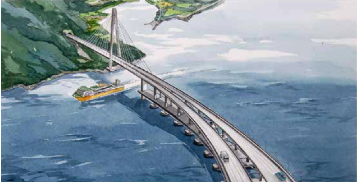
Figure 2.6: A suggestion of a floating bridge with end anchoring for Storfjorden (SVV, 2012a)
