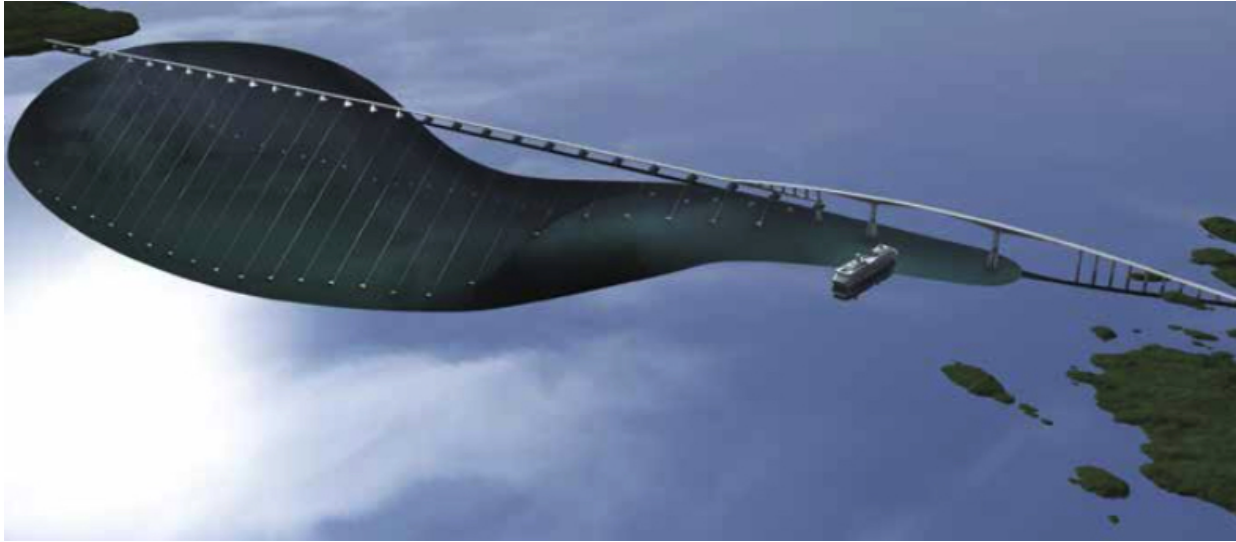
Figure 2.8: A suggestion of a floating bridge with side anchoring (SVV, 2012a)
