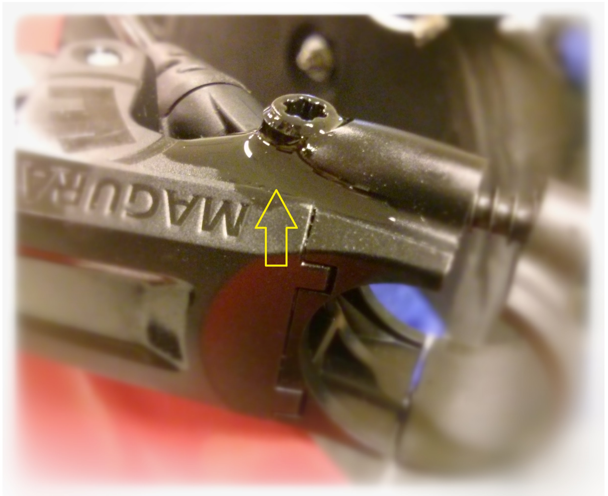
FIGURE E.4: Leakage around the lever bolt
