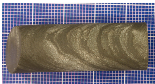
Figure 3-6 Heterogeneity of Mancos core plug ex. 1, dried with alcohol (Rugland 2014)
