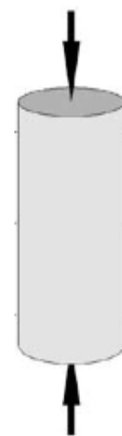
Figure 4-17 Axial Force applied. Zero confining pressure. Modified from (Fjær, et al. 2008)
