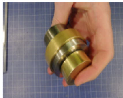
Figure 4-20 Used shale puncher, size and design. (Rademakers 2010)
