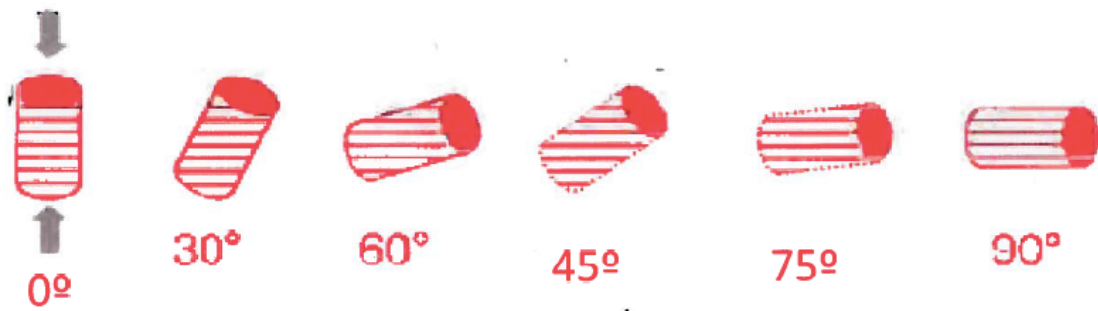
Figure 4-8 Orientation of drilled samples. Angle measured between the sample axis and the bedding plane normal. 0^\circ is situated normal to bedding plane, and 90^\circ is situated parallel to bedding plane (SINTEFPetroleum 2014).
