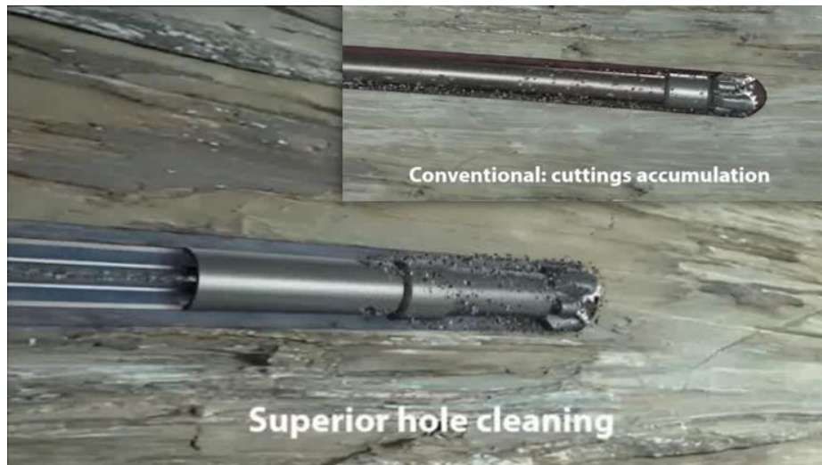
Figure 3-8 RDM cuttings transport (Reelwell AS u.d.)
