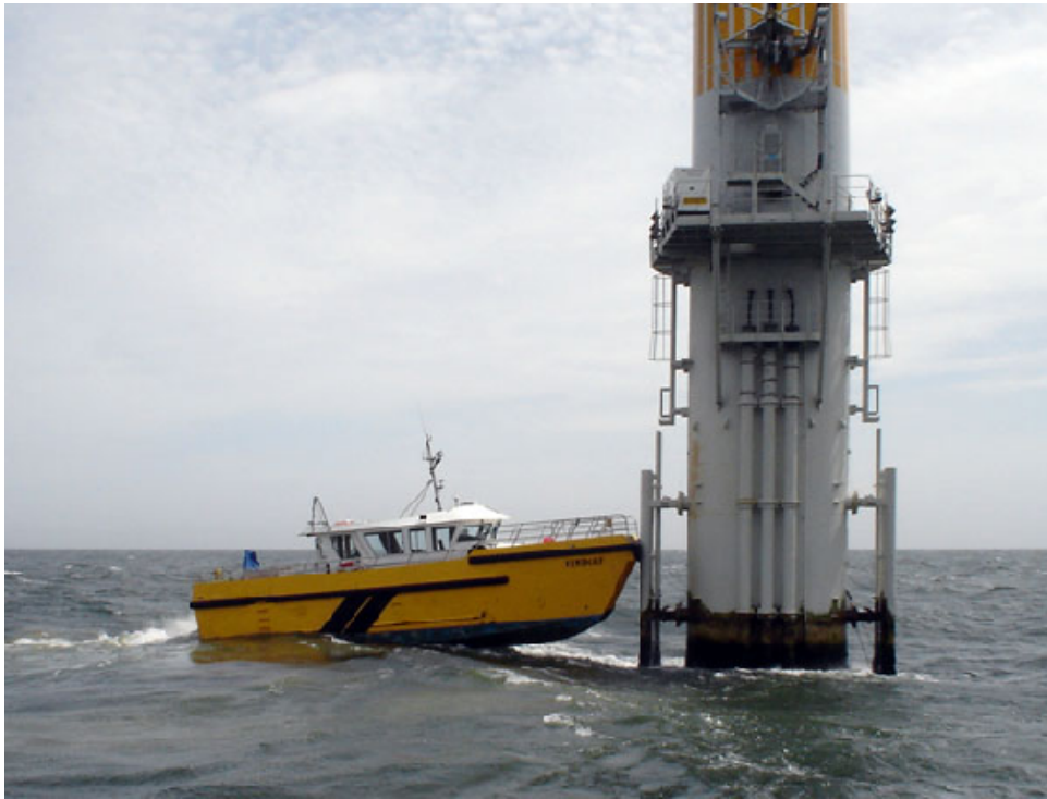
Figure 2.10: Fender docking, http://www.windcatworkboats.com/
