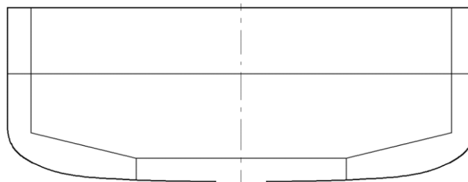
Figure 3-12: Cross section view of knuckled tank top (not used for any vessels in the study)
