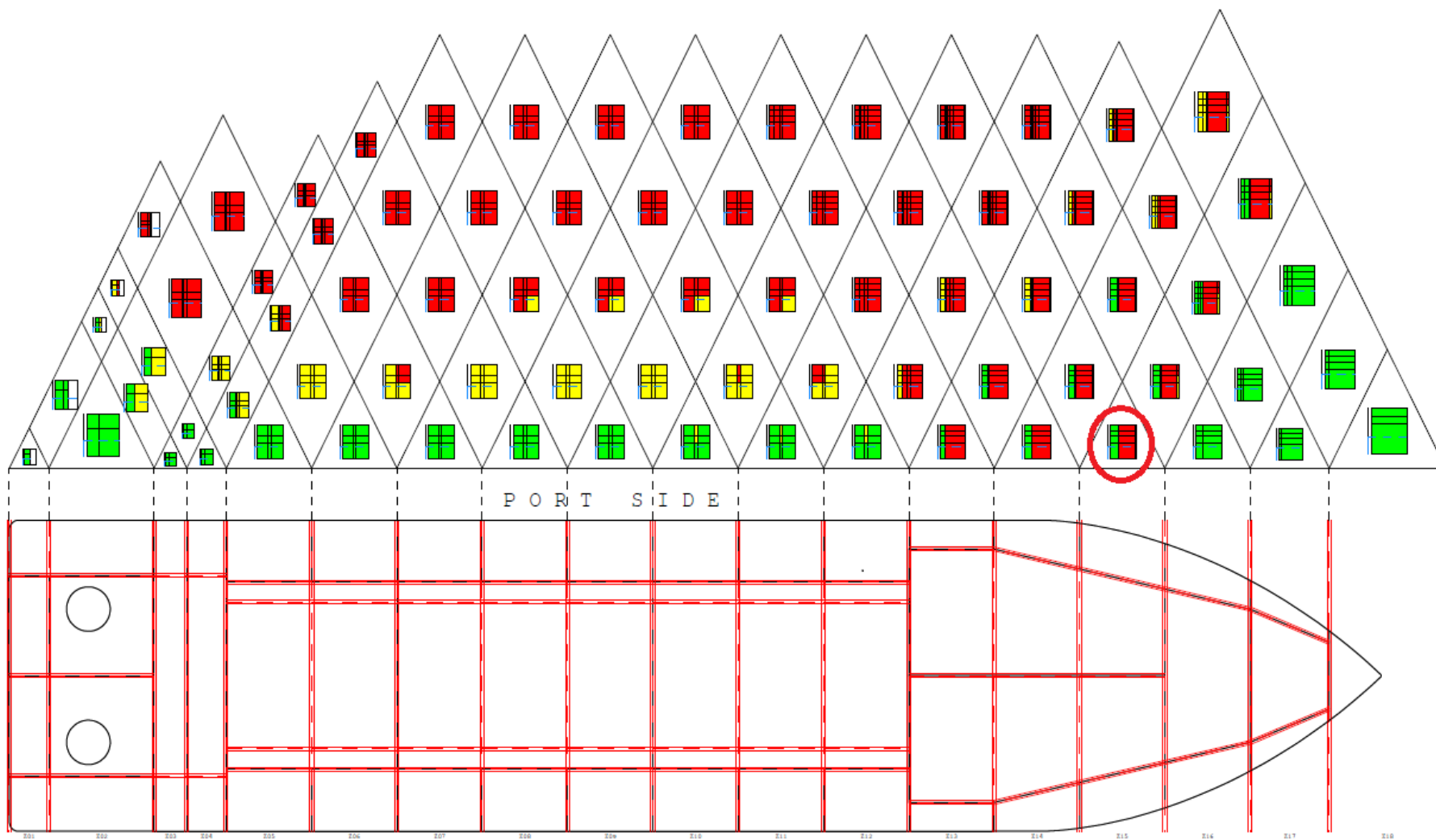
S-factor diagram for D 1 condition Vessel III, arrangement C
