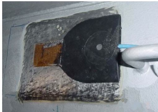
Figure 4.5: Sensor glued on stiffener before coating (Light Structures; 2009)
