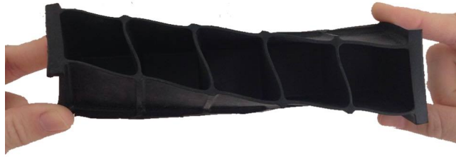
Figure 2.4: Torsion of an ice cube tray - an auxiliary model
