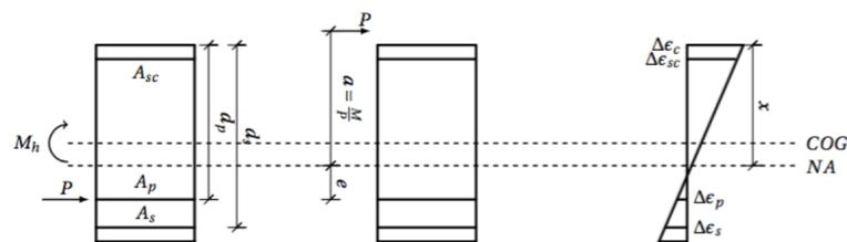
Either by increasing the amount of prestress or the distance  $d_p$ , this will lead to a relaxation of the loading introduced by the hydrostatic pressure. The compressive zone of the section, x, may then be manipulated so to fulfill requirements related to watertightness.
