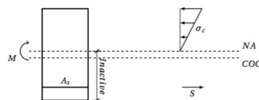
The illustration shows a cracked reinforced concrete section of a panel strip. An equivalent concrete moment of inertia may then be expressed according to [4] as:
