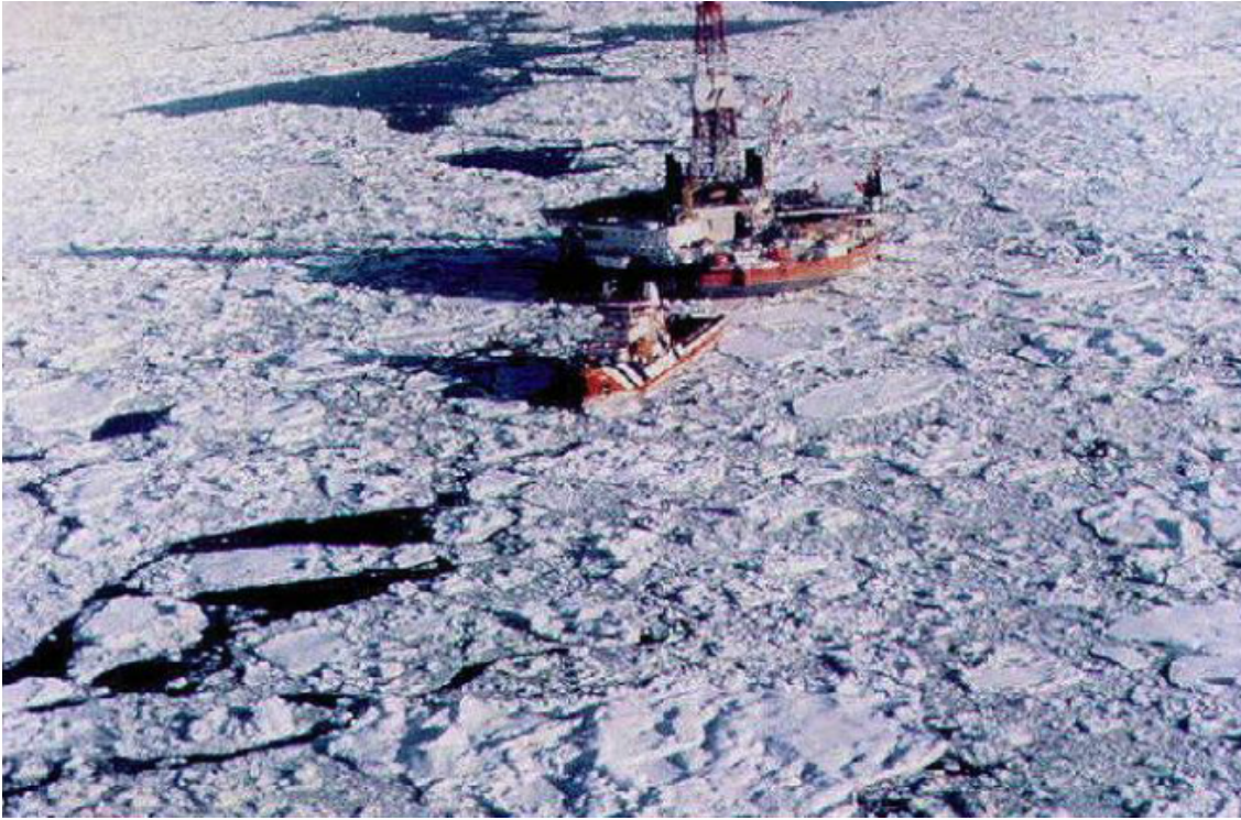
Figure 3.2: Kulluk in managed ice in the Canadian Beaufort Sea (Palmer and Croasdale, 2012).
