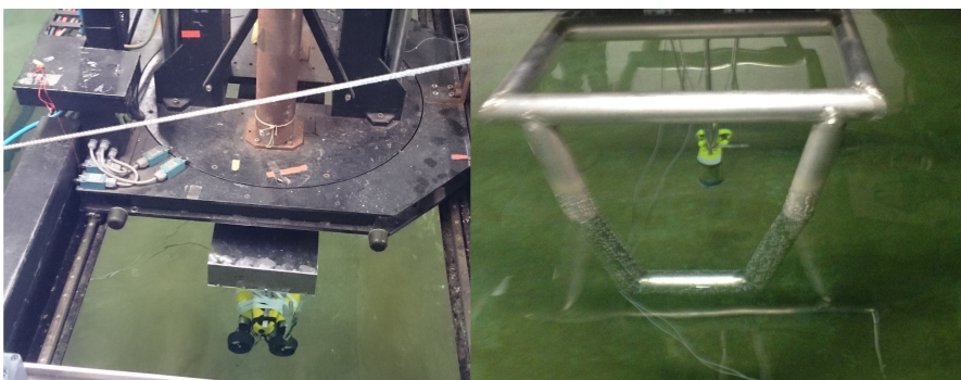
Figure 3.9: Towing test of VideoRay Pro-4(left) and Neptuneus(right)
