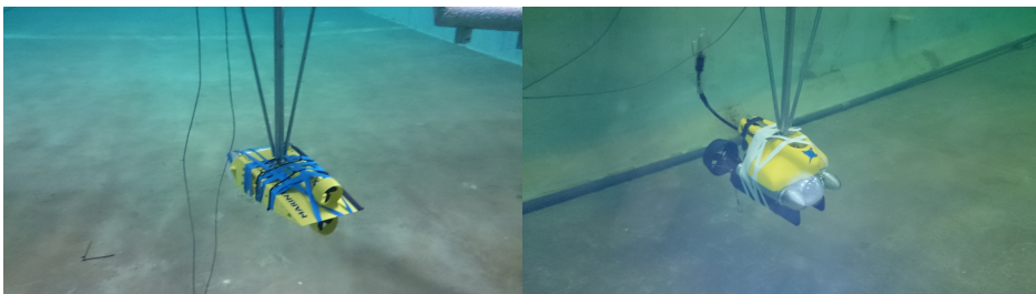
Figure 3.2: Underwater photos ROV Neptunus(left) and Videray PRO-4(right) mounted to bracket with strips, tape and screws for tests in heave/pitch(left) and surge/yaw(right).
