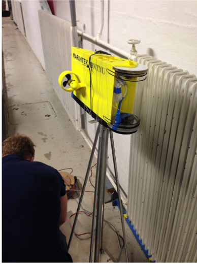
Figure 5: ROV Neptunus mounted for surge and yaw tests
