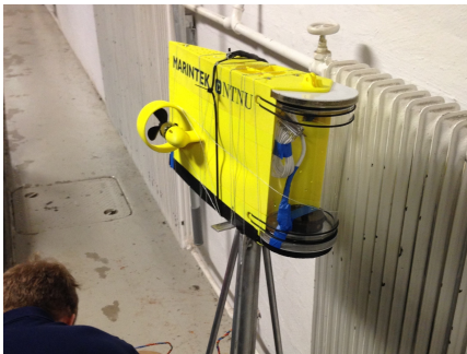
(a) ROV Neptunus mounted for surge and yaw tests)
