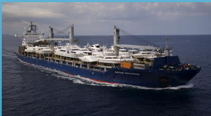
General cargo ships will have problems complying with the required EEDI. The ship type has higher cargo flexibility that leads to lower dwt/displacement ratio and has higher installed engine power to serve the shipping route with minimum delays.
