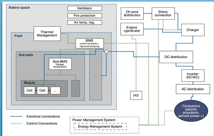
The figure above [4] represents a battery system with the different elements and systems around. The suggested solution is to install a lithium ion battery pack with high energy. Such a battery pack can supply the various propulsion loads, meaning both exploit the superfluous energy production and supplement the engines when energy demand is high. Results from case study and the economical study will not be presented here, due to state of the work progress.
