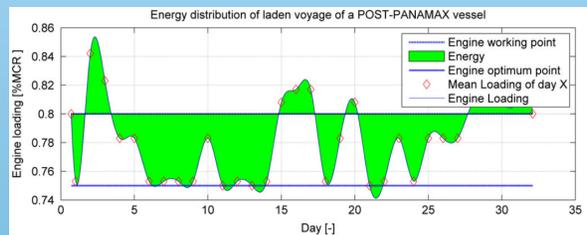
The graph [3] shows an engine loading curve for a ship in laden voyage. The green area indicates the fluctuations, day by day, from the engine optimum point. This can be served by a hybrid battery system and the engine can always work on optimum point. This results in less fuel consumption and hence less emissions from the engines.
