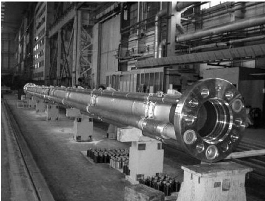
Figure 7: Aluminum drilling-riser joint with peripheral lines [16].
