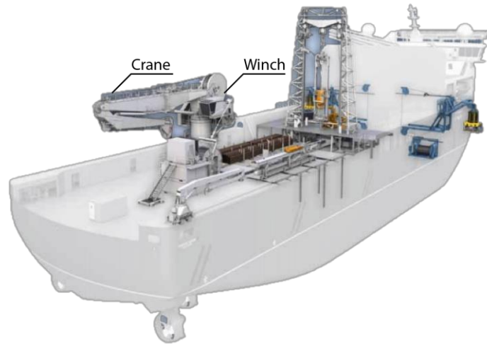
Figure 2.1: OSCV with Elevated Crane Winch. (Roll's Royce)
