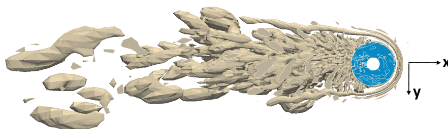
FIGURE 5.18: 2D view of instantaneous vortical structures around the circular GBF at t = 109.8 \frac{D}{U_\infty} , seen in the positive z -direction
