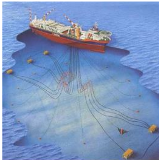
Figure 1-1 Turret-moored production ship - Norne FPSO (Larsen K. , 2014)
