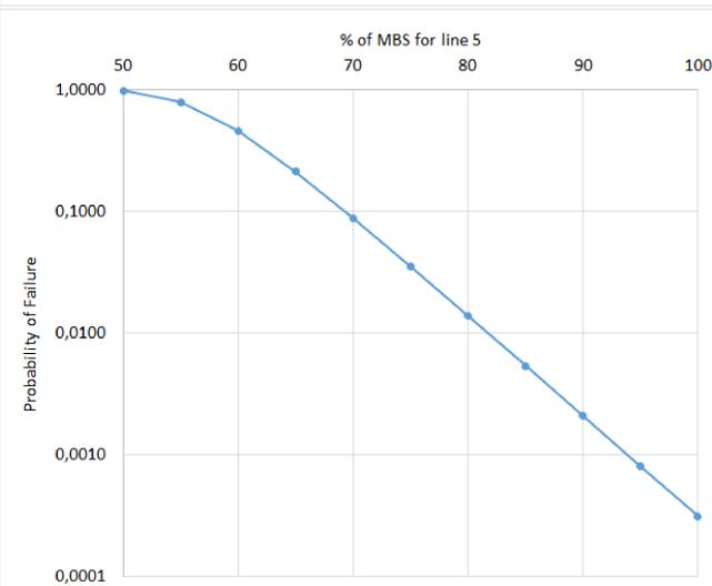
The graph shows the probability of failure as a function of MBS, when one line is already broken. When the MBS is 100%, which is reasonable, there is only a 0.03% chance of failure. With a degradation of MBS to 80%, there is still just 1.38% chance of progressive collapse. This shows that the mooring system has a high redundancy, and is robust even with one line broken.
