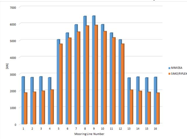
The figure to the left shows the maximum tension in all sixteen mooring lines, with contributions from SIMO/RIFLEX and MIMOSA. As the figure depicts, the maximum tension comparison is acceptable, with 9.4% deviation in the most loaded line. The results from MIMOSA are conservative, which is expected due to the linearisation and excluding of damping contribution.
