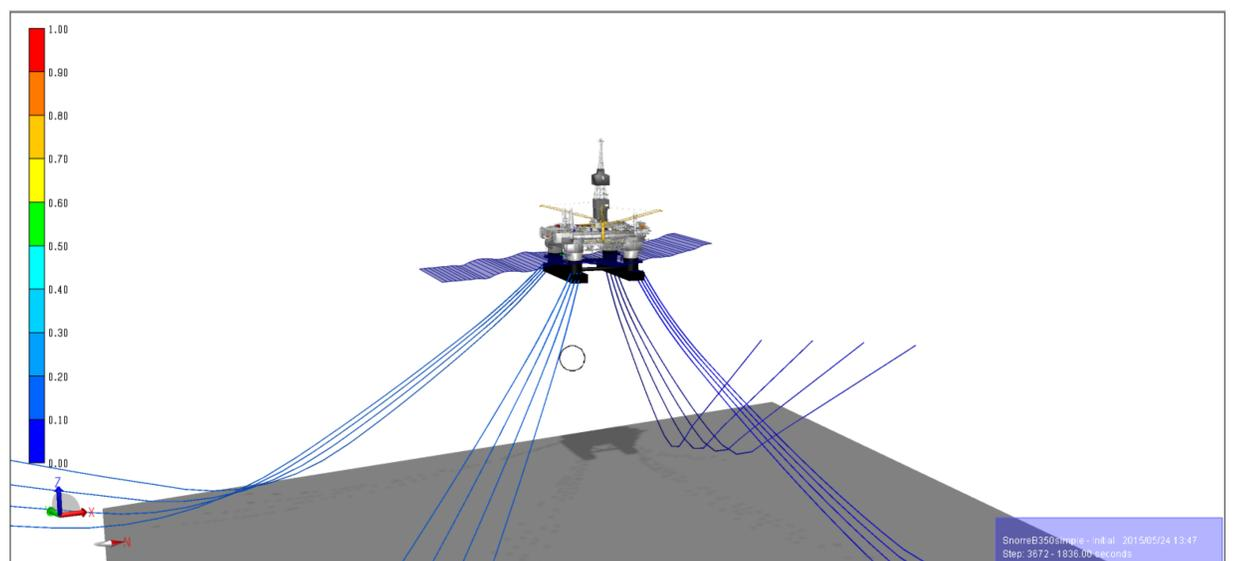
The model analysed was the Snorre B semi submersible platform, with 16 mooring lines grouped in four clusters. A picture of the SIMO/RIFLEX model, displayed in the SIMA GUI, is shown above.
