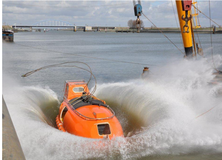
Figure 5.3: Impact during drop test of a conventional lifeboat, (Safety, 2015)
