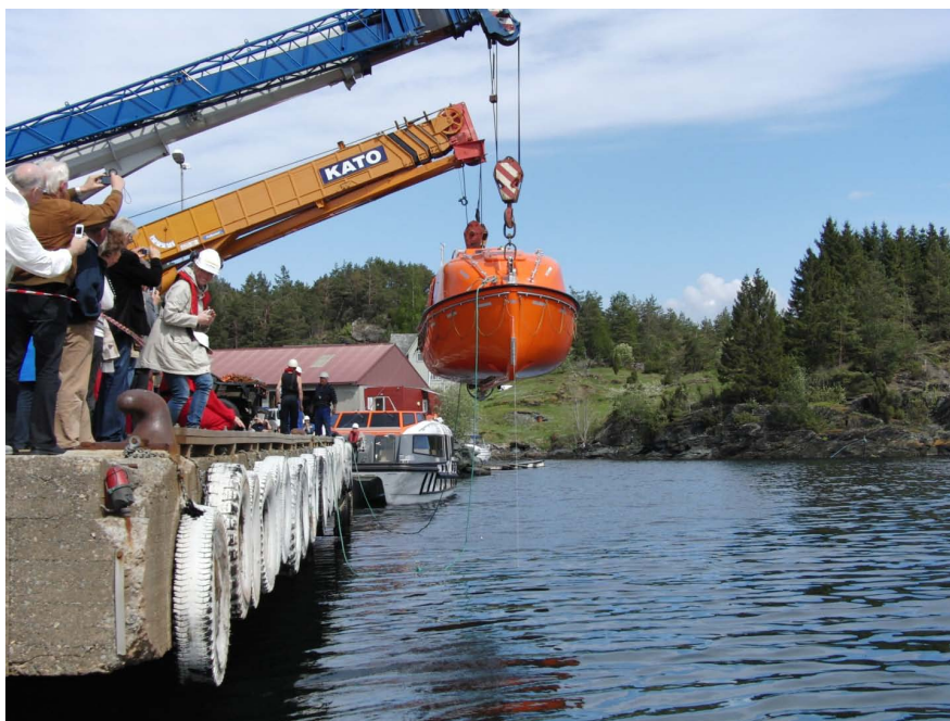
Figure 5.2: Lifeboat prior to free-fall drop of 3 m, (Marintek, 2011)
