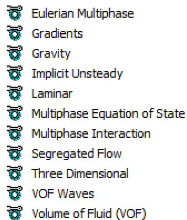
Figure 5.16: Selected physical modules for rigid CFD analysis
