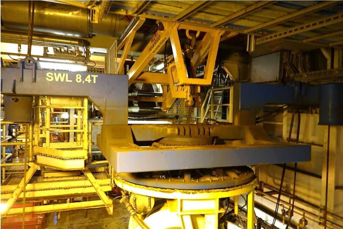
Figure 2.4: The blue cursor frame on top of the TMS illustrating clearance to the sheave.
