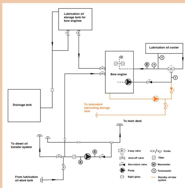
Figure 1. System illustration of lubrication oil system.
