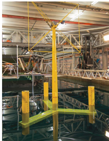
Figure. 1.5 5-MW-CSC substructure model test at scale 1:30. MARINTEK [17]
