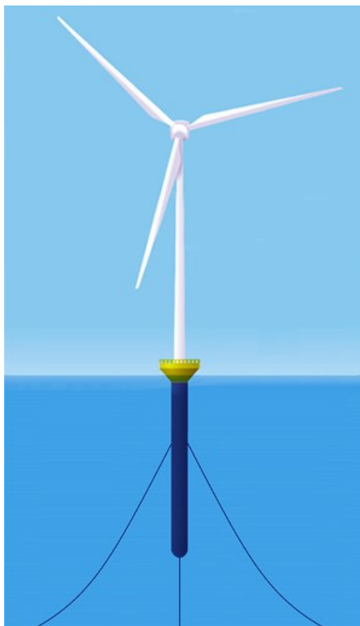
Figure 3.1: Phase IV – Floating spar buoy described in the Offshore Code Comparison Collaboration (OC3) for IEA Task 23. In the model Phase IV – Floating spar buoy, NREL offshore 5-MW wind turbine is installed on a floating spar-buoy in deep water (320 m) (from http://www.hawc2.dk )
