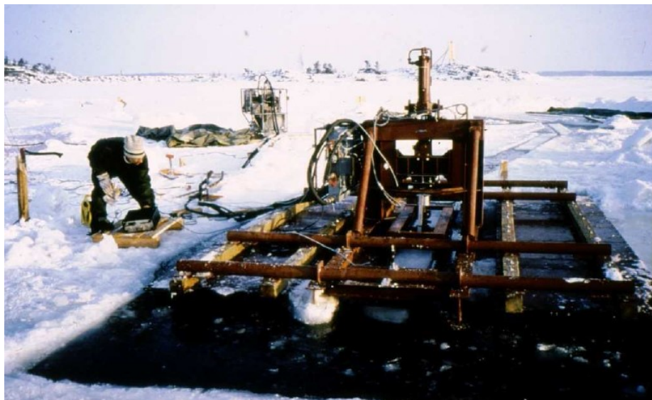
Figure 2.9: Ice flexural strength measurement (Kujala, 2013)
