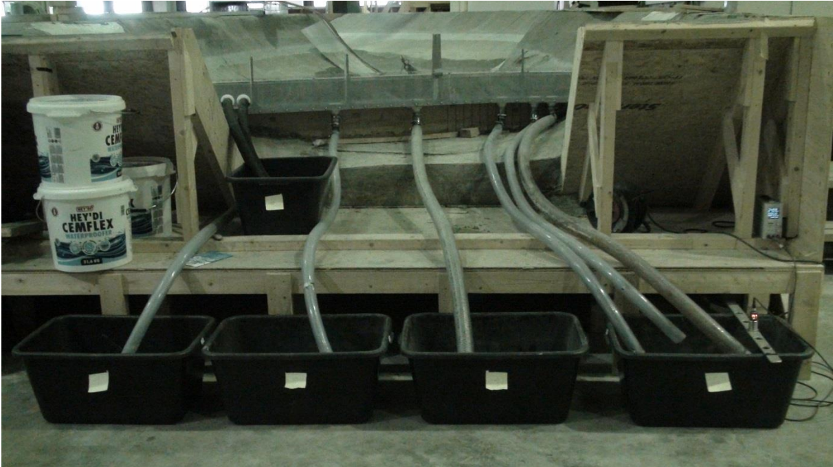
Figure 3-8 Collection buckets and outlets
