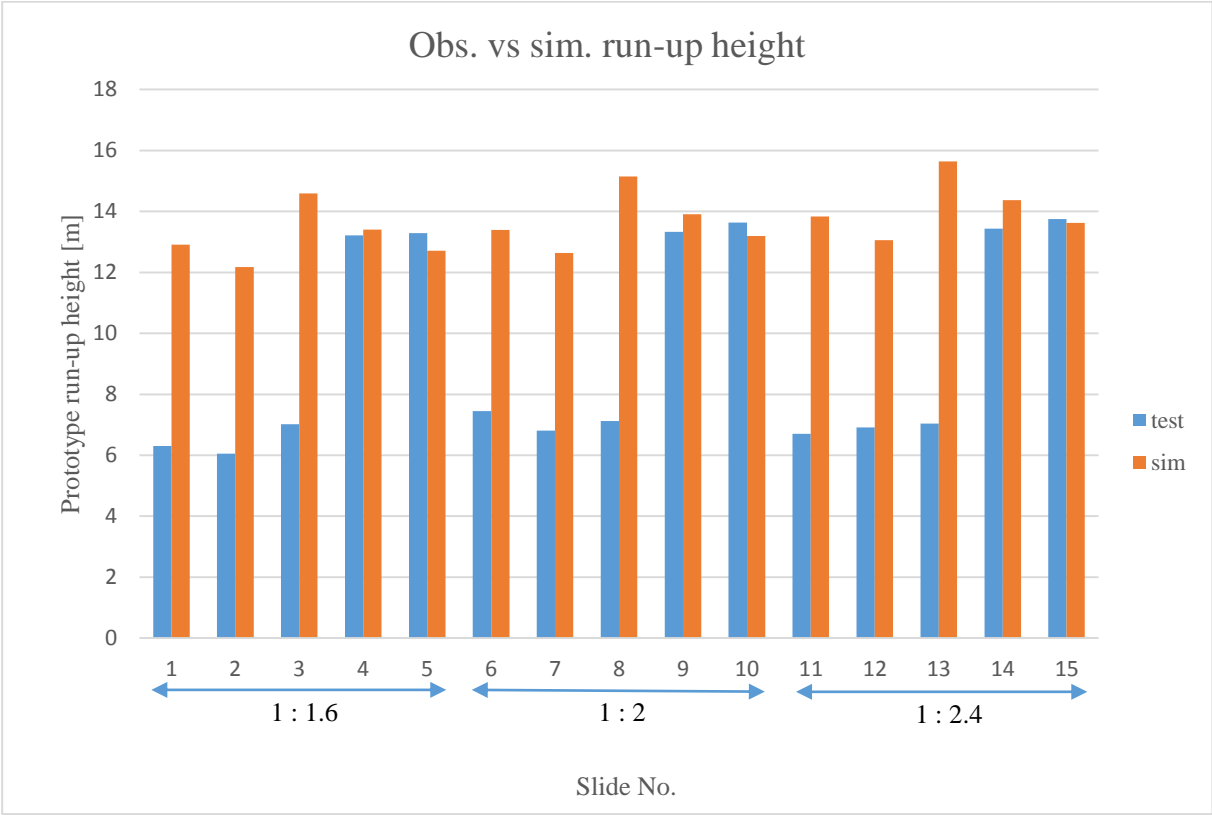
Figure 6-3 Comparison between observed and simulated run-up height
