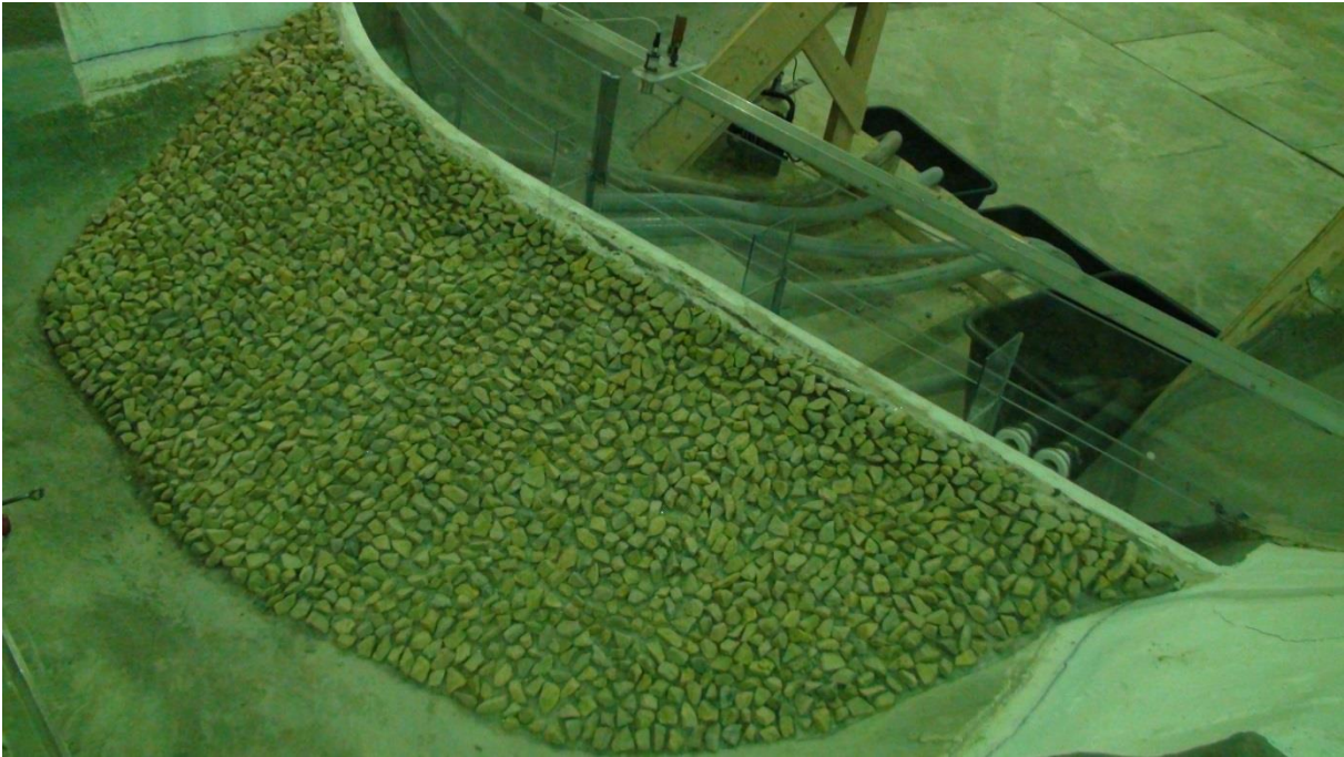
Figure 3-6 Dam structure with increased roughness
